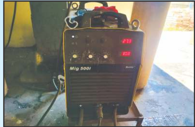
MAKE:- ESAB/GAIGU/MOGRA/SUNRISE/PANASONIC CAPACITY/RANGE:- 400 Amps/500 Amps MODEL:- MIG400 CCCV, SNER-500M MACHINE No:- 19074400490 YEAR OF BUILD:- 2009-2019
