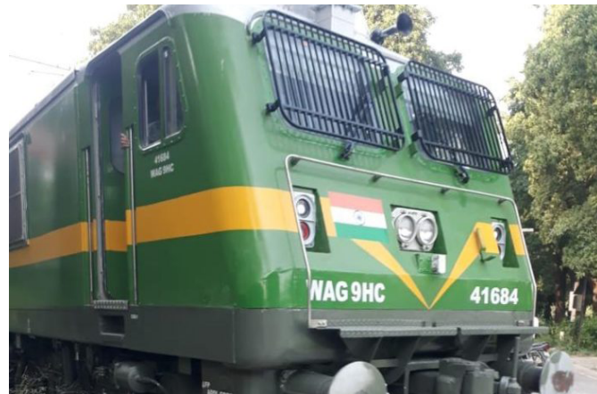
Complete Shell Assembly
